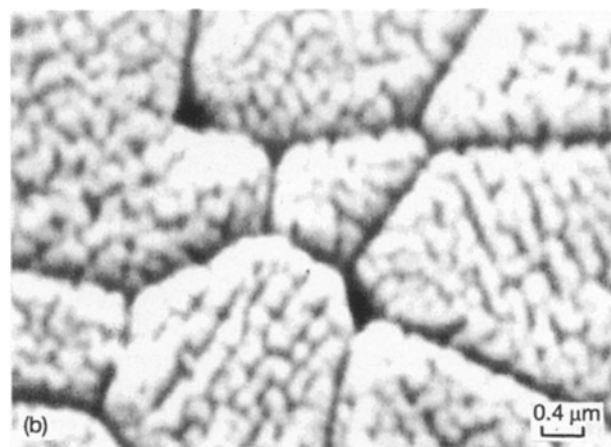
Figure 12b SEM micrographs showing the sintered structure for material 2. The sintering times were 30 and 120 min for (a) and (b) respectively.
